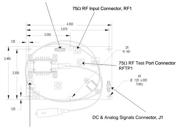
$50\Omega$  RF Input Connector, RF2 (if applicable)
