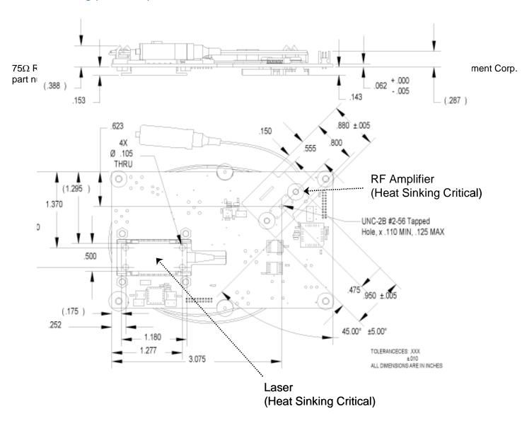
$75\Omega$  RF connector – MCX connector, straight jack receptacle, Koaxis part number 253-5700, or General Instrument Corp. part number 404576-001-99.
